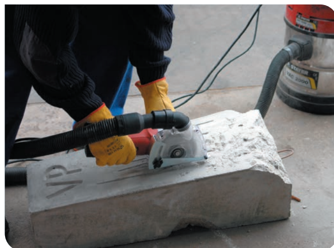
CUTTING WITH AIR SUCTION PROTECTION GUARD.
